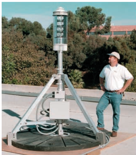
AirFiber's OptiMesh rooftop node supports a mesh network of wireless optical links.
