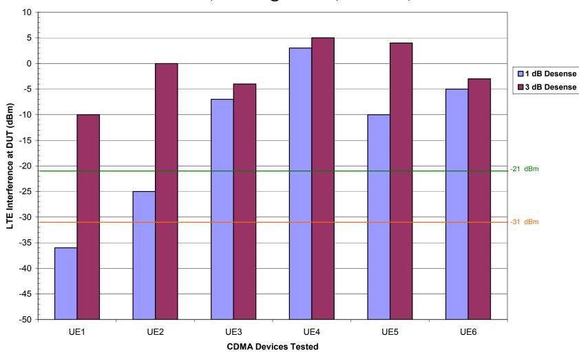
Receiver Blocking Test Results CDMA DUT Ch. 25, LTE 3MHz @ 1916.5MHz, PUSCH 4RBs, Offset 10
