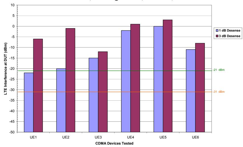
Intermodulation and Receiver Blocking Test Results CDMA DUT Ch. 550, LTE 5MHz @ 1917.5MHz, PUSCH 1RBs, Offset 13
