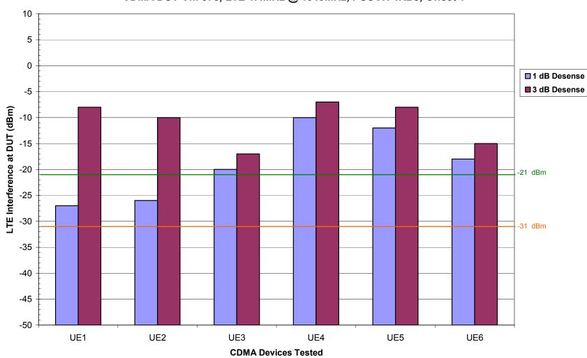
Intermodulation and Receiver Blocking Test Results CDMA DUT Ch. 575, LTE 1.4MHz @ 1919MHz, PUSCH 4RBs, Offset 1
