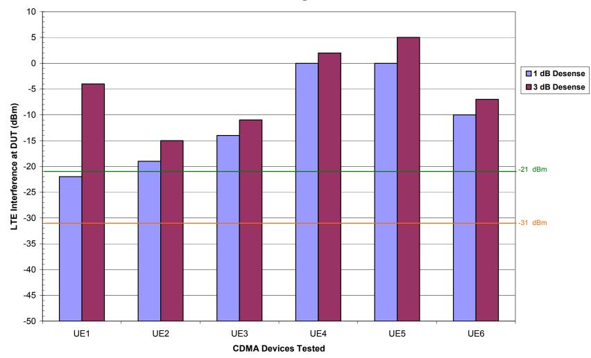
Intermodulation and Receiver Blocking Test Results CDMA DUT Ch. 550, LTE 3MHz @ 1916.5MHz, PUCCH RB0/14
