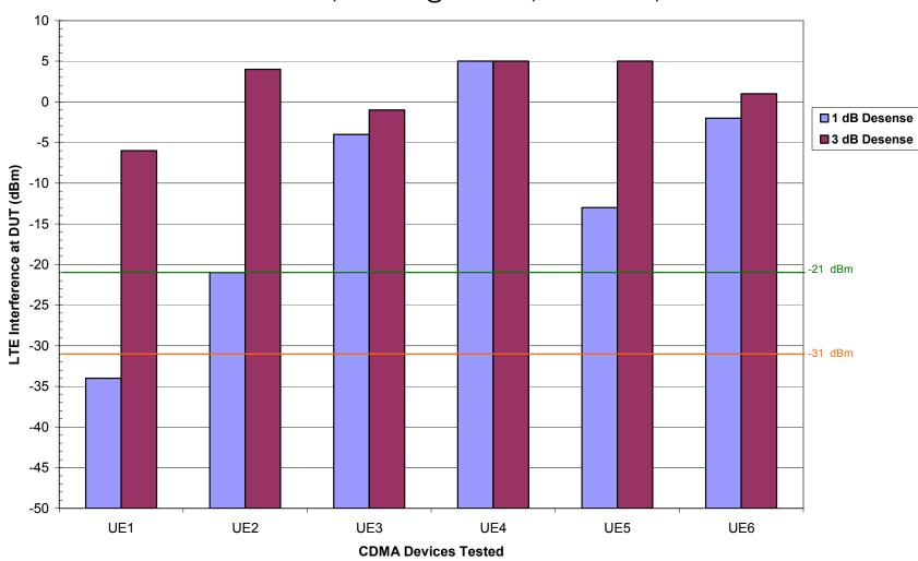
Receiver Blocking Test Results CDMA DUT Ch. 25, LTE 3MHz @ 1916.5MHz, PUSCH 13RBs, Offset 1
