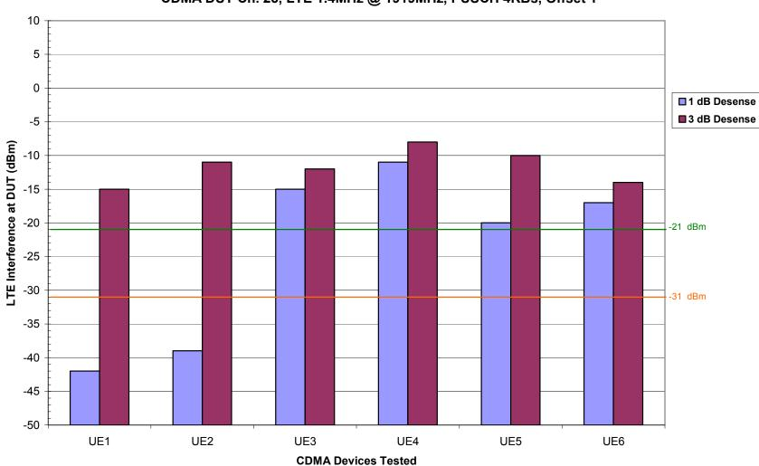
Receiver Blocking Test Results CDMA DUT Ch. 25, LTE 1.4MHz @ 1919MHz, PUSCH 4RBs, Offset 1
